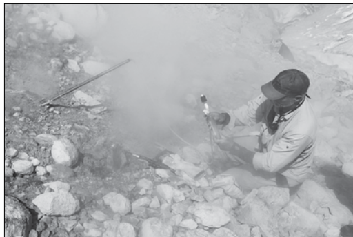
Gases from a fumarole in Mount Baker's Sherman Crater are collected by Western's Dave Tucker, using vacuum flasks, a titanium tube and heat-resistant tubing, for later analysis on campus. Tucker presented a history of Mount Baker at the Whatcom Museum of History and Art.
